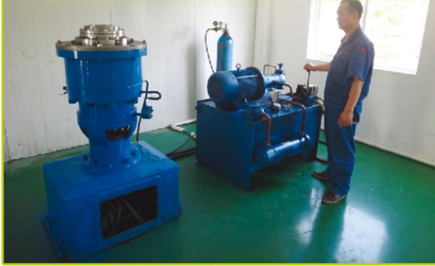
Mechanical Seals for Kettles Testing Platform 釜用机械密封测试平台
