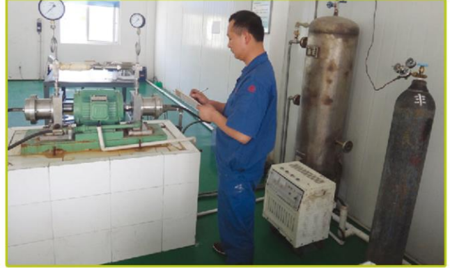
Mechanical Seals for Pumps Testing Platform 泵用机械密封测试平台
